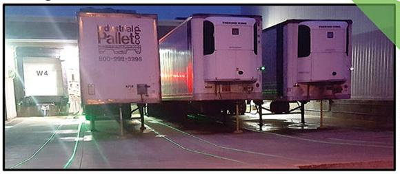
This is why Laser Tools Co.'s Laser Docking™ System is the perfect trailer docking assistant. A driver can "see" the laser docking lines in his wing mirrors when the truck and trailer are approaching the docking lane. This guides the driver while backing up to the loading dock. Also, the laser lines provide a visual indication that the trailer is centered to the loading dock.
