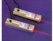
Model 58 Alignment Module. 2 1/2" L x 3/4" Diameter. Specs.: Dimension: 3-12VDC regulated 50ma. Power: Laser Beam: 635nm Class IT or IIIa.
